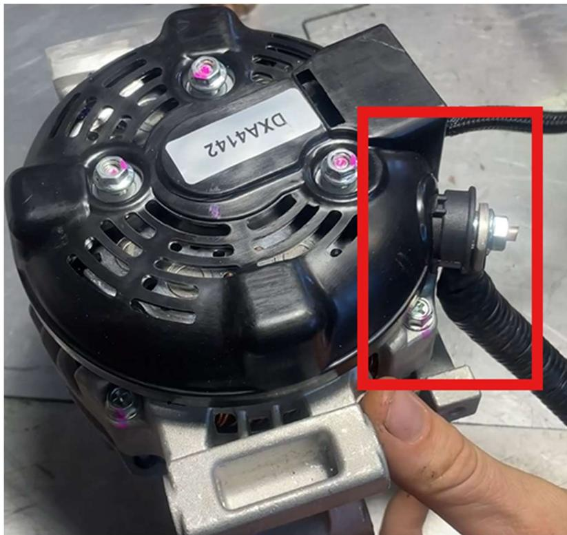
Remove the protruding bolt lug from the body of the alternator. This lug needs to be cut off to allow the alternator to fit in its new location. Removing this lug does not prevent the alternator from being mounted in the factory location. When removing the lug it is important to wrap up the alternator to prevent cutting debris from damaging the internals of the alternator.
