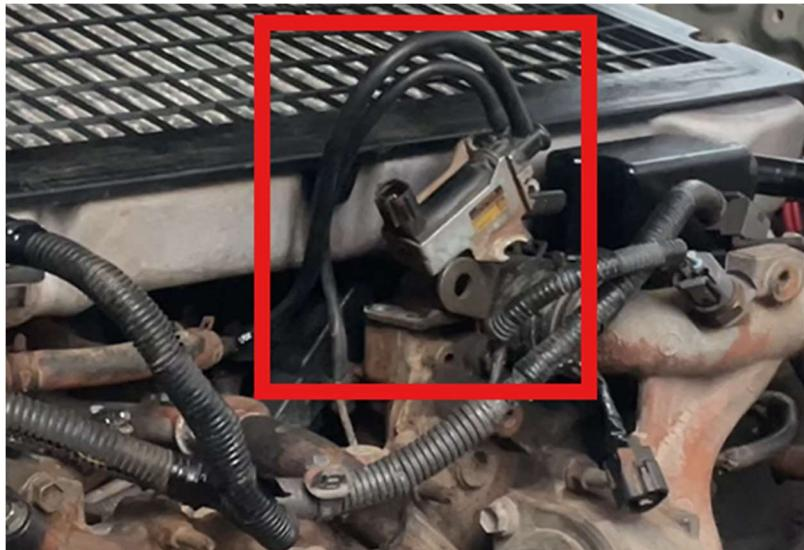
7. Unbolt Coolant pipe under intercooler and extend perpendicular adjoining hose with supplied hose, barb and hose clamps.
