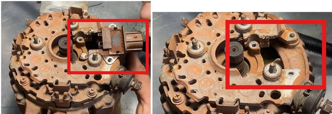
Install the Bakerlite brace piece as shown in the back of the alternator. Re-install the brushes and mount the left hand tab of the brush housing to the bakerlite brace piece. This will hold the brushes in place.
