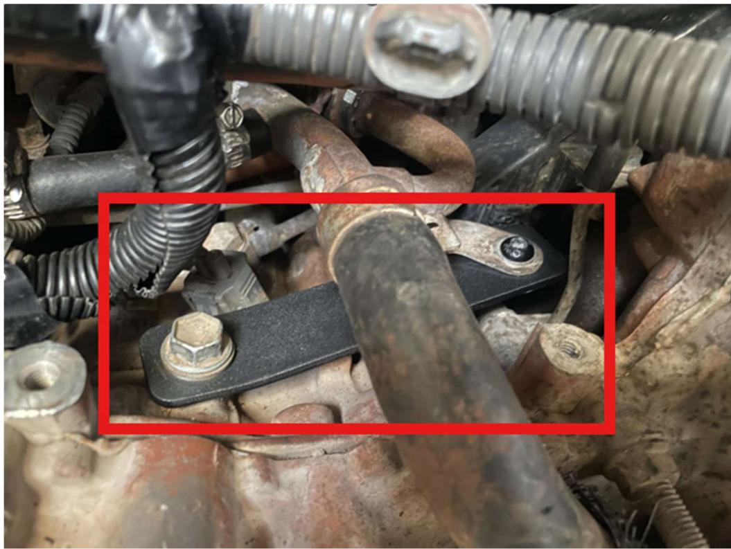
Using the supplied part pictured and an M6 cap screw, washer and spring washer, mount the coolant pipe in the new location as shown. Low to Medium strength thread locker may be used if desired.
