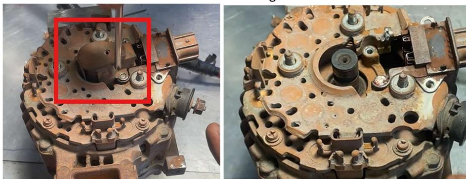
Remove the voltage regulator from the alternator by first removing the screws, taking note of where they went, and then using a soldering iron to melt the soldered connection. If an upwards force is applied to the regulator whilst the connection is being heated, when the solder melts the regulator will come free.
